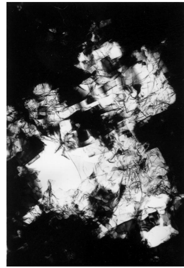
Figure 9 Transmission electron micrograph of master alloy Al-2 wt% Sr ribbon.
